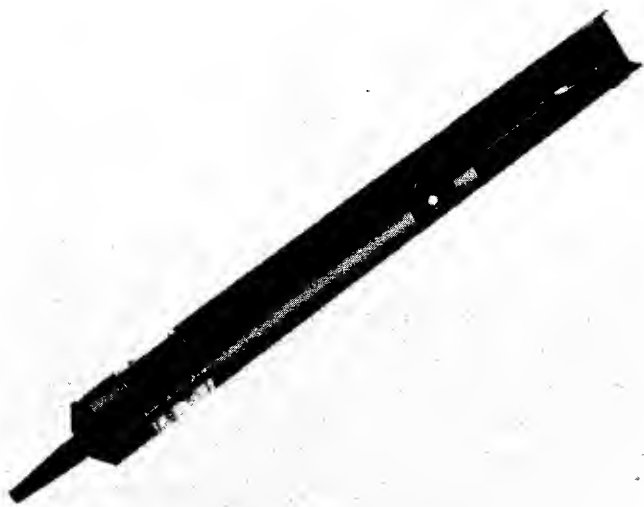
Fig. 6-25. The spring-driver plunger in the solder vacuum pump is used to pull hot solder off a connection.
